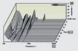
ABOVE: Cumulative resonant decay spectrum, illustrating various bearing housing, pillar and arm vibration modes spanning 100Hz-10kHz over 40msec
